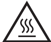
Caution, hot surface
